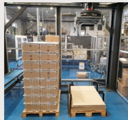
The 4-sides open version gives the possibility to increase the number of bays, even with an interlayer or empty pallet storage.
