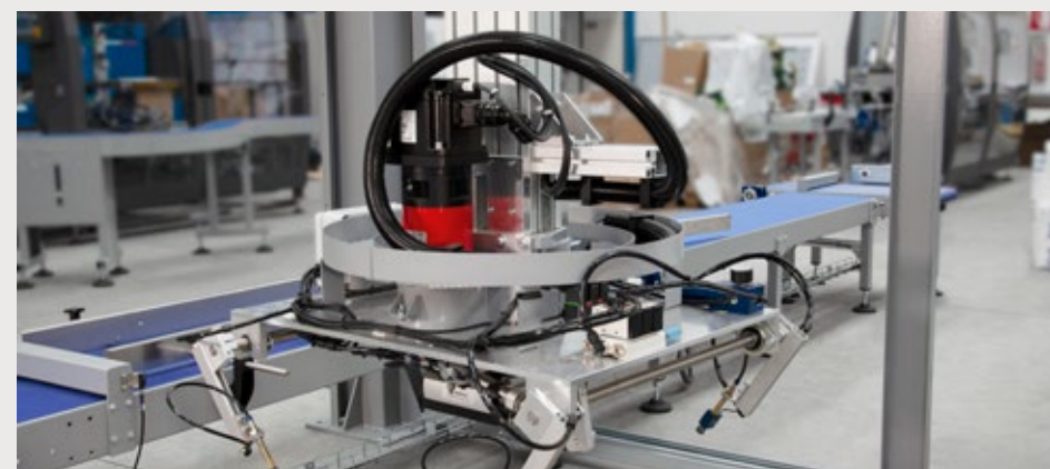
Various types of gripping modules (possibility of automatic quick coupling and release).
