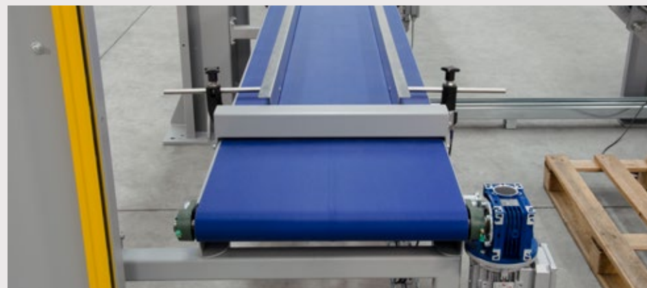
PALLETIZER infeed belt equipped with optical sensors for products' reading. At this station, products are accurately presented at the picking station.
