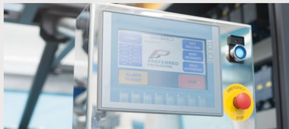
User friendly OMRON touch screen, with recordable programs menu system recipe based. Most of format changes and movements are electric and can be recorded and recalled. Machine can be accessed from both sides.
