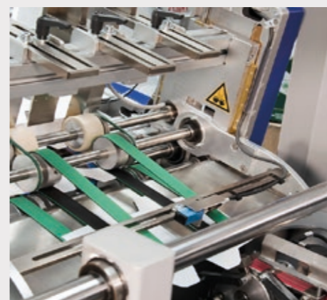
Blanks warehouse with precise release mechanism, precisely synchronised with the arriving product, equipped with a photocell indicating boxes almost finished.
