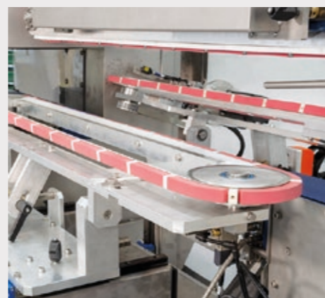
Output station with guide belts adjusted to the width of the box.
