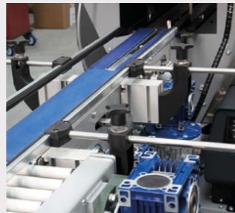
Infeed belt designed to product measurement, can be connected to previous line
