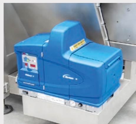
Hot met glue applicator to close the lower flaps by Meler, Nordson or Noxon, on the client's request.
