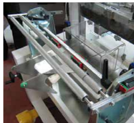
An adjustable tunnel allows the packaging of a lot of different kind of products with wide range of measures.
