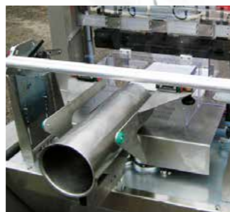
Machine can optionally be equipped with an in feed loading pipe for easy products loading.
