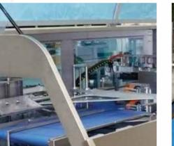
Side sealing machine 3 belts for products
