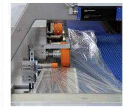
flat film . NO premade bags. Machine works in conveyor (depending on the products type)
