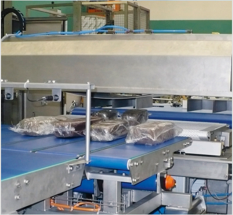
Packaging machine and vacuum chamber connected using belts or diverters, based on the client's requirements. Customised, made-to-measure layout.
