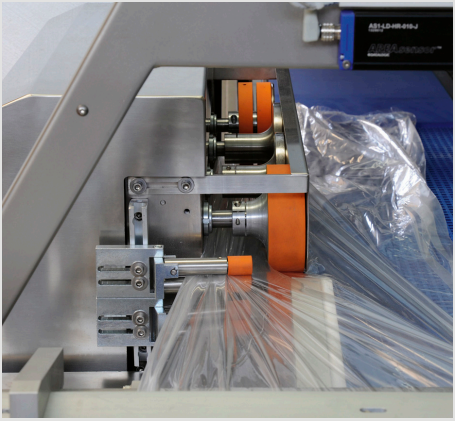
Intralox conveyors for food or smooth belts which are easily dismantled (based on the product) excellent for cleaning.
