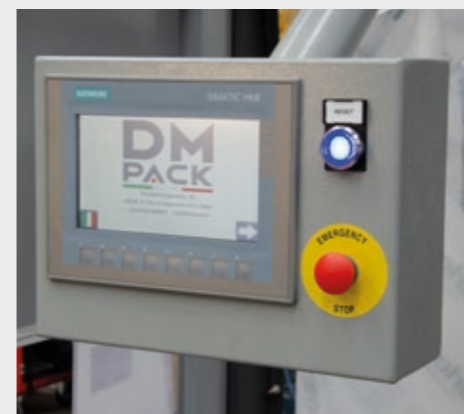
Touch screen for convenient operator interface when reading and programming machine parameters. Saves up to 25 different programs.
