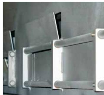
The flaps could be opened and also adjustable for a best ventilation, accordingly the best shrinking.
