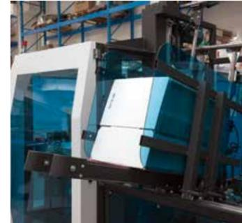
Blank picking system provided with motor.
