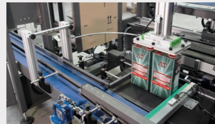
Pick and place system for fast & accurate products picking up from the infeed transport conveyor and precise feeding of the carton with the configuration previously set.
