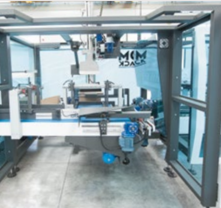
Completely accessible and openable. Separable loading and cartoning stations to allow operator's access for easy maintenance.
