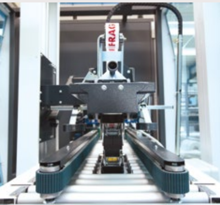
Out feed station with motorised driven belts adjustable to different carton sizes.
