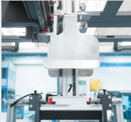
Pick and place system for fast & accurate products picking up from the infeed transport conveyor and precise feeding of the carton with the configuration previously set.
