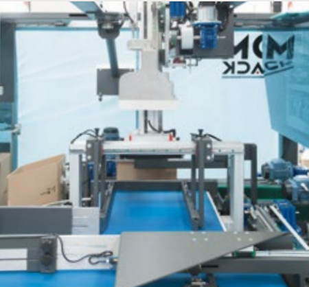
New generation case packer machine. Compact, automatic, equipped with an easy change of format and motorized adjustments.
