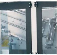
Precutting device for carton & carton's Double dispenser unit for adhesive tape. stock.
