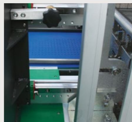
All movements on linear Hiwin guides.
