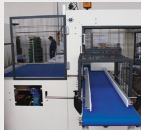
The machine can be equipped with in line or 90° conveyor with pusher for higher speed, and for automatic multipack forming.
