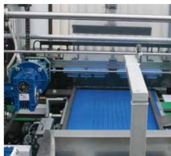
Motorized Sealing bar & pusher.
