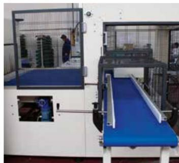
The machine can be equipped with in line conveyor; 90° conveyor with pusher for higher speed, and for automatic multipack forming.
