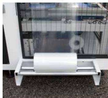
Both film roll in lower position for easy load.
