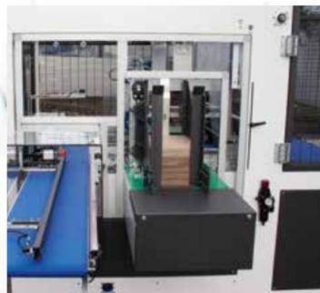
90° automatic grouping & feeding version. Different layout can be done for products feeding from left or from right.
