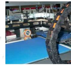
The L vertical bar which guarantees the Bar width just 1 cm, vertical movement same pressure on the film welding replaand not scissor, uniform sealing, low film alone L sealer separted from the tunnel.
