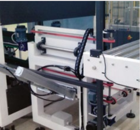
Machine controlled by Omron PLC and intuitive touch panel. Auto-adjustable change of format.
