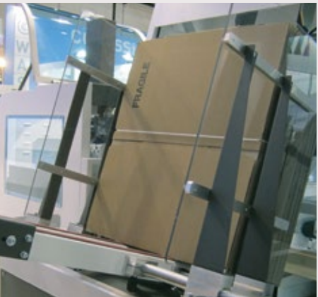
Blank picking system provided with motor.
