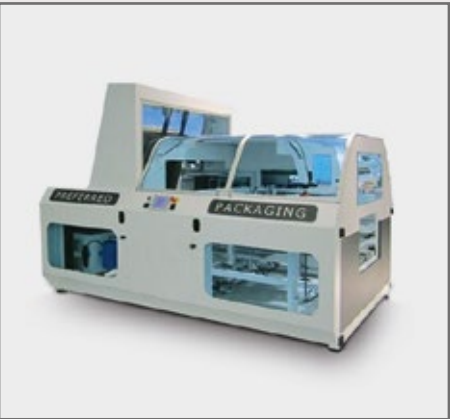
Automatic case closing with tape(as optional with hot melt). Motorised side guides.
