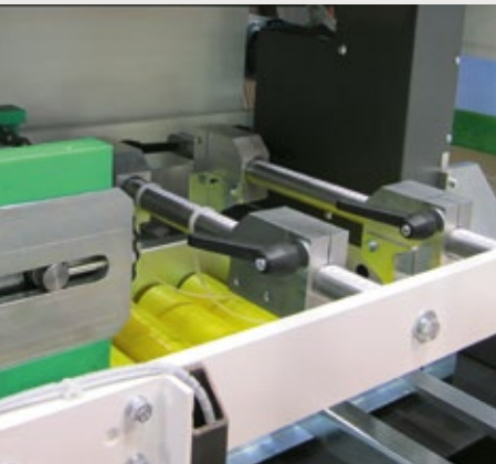
In feed conveyor with different loading systems depending on the products.
