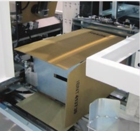
Automatic cartons opening and products insertion.
