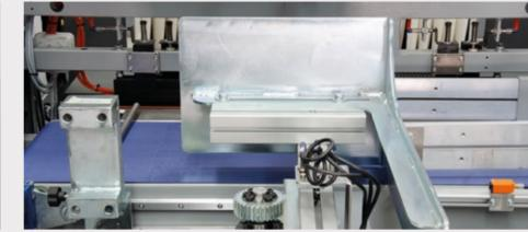
Also available in a compact version with a built- The machine can be equipped with a 90° belt and pusher for greater speed and automatic grouping.
