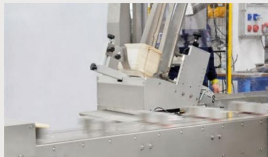
Transport Conveyor designed based on product sizes, available in different versions: in sectors, with regular belt
