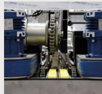
Motorized side belts that ensure stability to the product in the output even at high speeds
