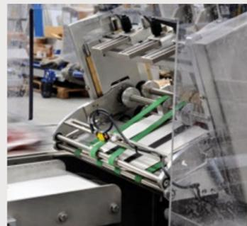
Precise and effective release system of the cartons from the warehouse, in the continuous version, or by means of a motorized arm equipped with suction cups in the intermittent version
