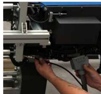
Easy connectors for each part to reduce working and stop timing. Operator's manual working.
