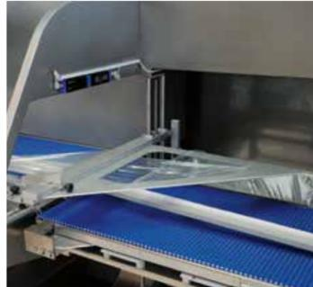
Film inverting head –triangle for center folded or flat film . NO premade bags. Machine works in line with film roll. High versatility and film costs saving.
