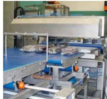
Packaging machine & vacuum chambers can be connected by conveyors, dividers depending on customer's need. Customized layout.
