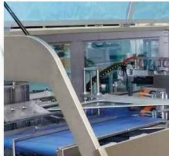
Side sealing machine 3 belts for products wrapping before vacuum. Strong air tight sealing.
