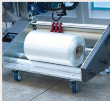
Extractable film dispenser unit. For easy film threading & quick change. Machine usually works with center folded film; it can also work with flat film as an option.
