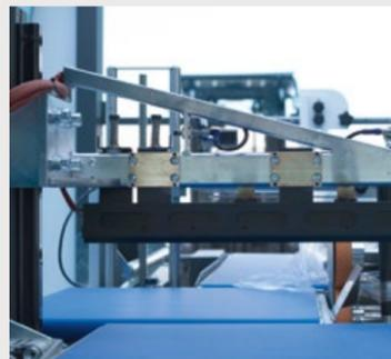
Movable central conveyor allows products to always run in the center. No need to move the shrinking tunnel or the infeed conveyor.
