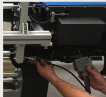
Connectors allow a fast connection to reduce operator's working time.
