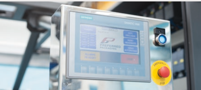
Intuitive touch screen for simple format change. The touch screen can rotate in 3 different positions to allow the operator to work on all sides of the machine, front, back and side.
