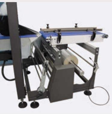
Film dispenser unit with single or double film rolls with joined seal bar for fast film change.
