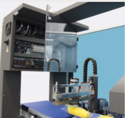
Electric box on view, positioned up high, perfectly accessible for the operator.
