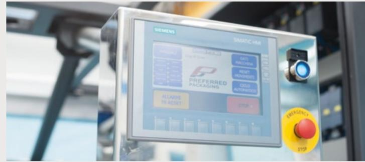
Intuitive touch screen for simple format change. It can rotate in 3 different positions to allow the operator to work on both sides.
