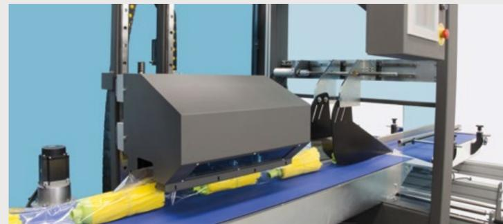
This flowpack machine is equipped with a top sealer (reel from the bottom).
