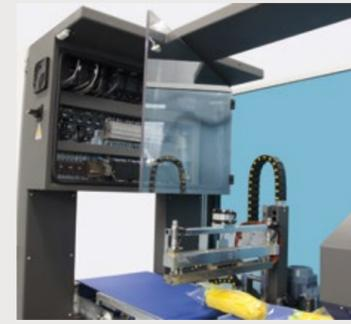
Electric panel on view, perfectly accessible to the operator thanks to its high position.
