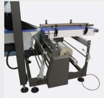
Single film dispenser unit as standard; double film dispenser with sealing bar for a fast film change as optional.
