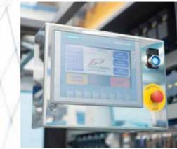
Touch screen intuitive and for easy change of format. Touch screen can rotate in 3 positions. Operator can operate and access the machine from the FRONT/BACK & SIDE. Machine is left/right.
