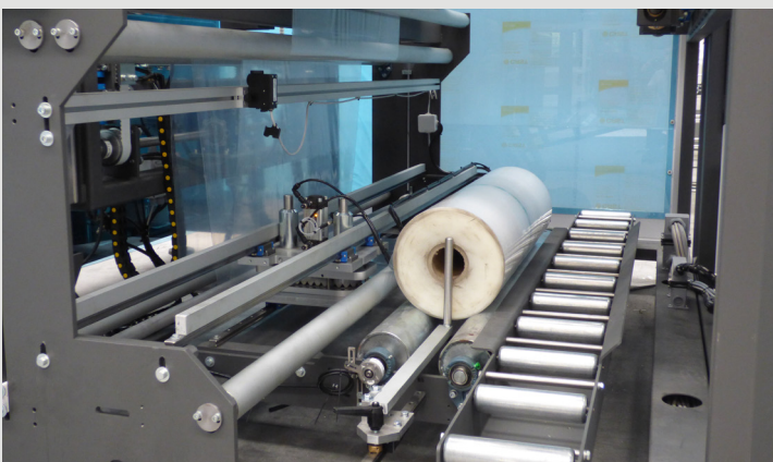
Cantilever and accessible from both sides. Reel holder with trolley for facilitated loading and replacement.
