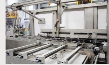
Row of motorized pushers that allow a precise and continuous insertion of the product inside the box
