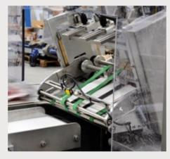
Precise and effective release system of the cartons from the warehouse, in the continuous product in the output even at high speeds version, or by means of a motorized arm equipped with suction cups in the intermittent
