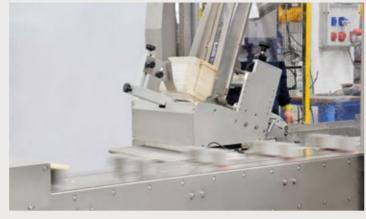
Tansport Conveyor designed based on product sizes, available in different versions: in sectors, with regular belt
