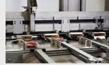
Mechanical flap opening, upper belts that allow safe and stable transport of the carton to the outfeed station
