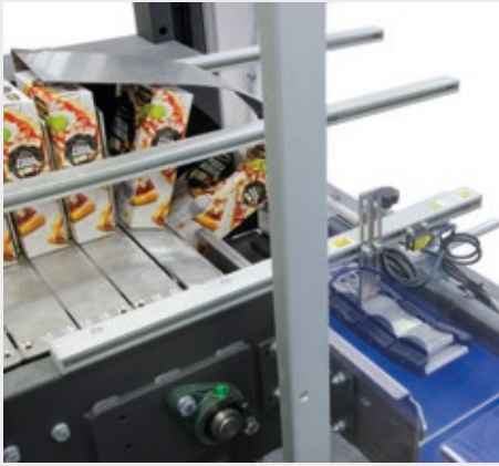
Flexible infeed belt, adjustable for different products size and grouping configurations.
