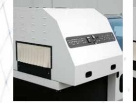
The chamber of the shrink tunnel can be horizontally moved thanks to the frontal handles Easy controls for speed, air and temperature to be always centered with the incoming products, coming out from the sealing machine adjustments. in order to obtain a perfect shrinking even without moving the complete shrink tunnel with forklift.
