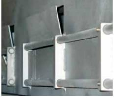
The flaps could be opened and also adjustable for a best ventilation, accordingly the best shrinking.
