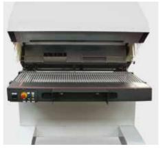
Opening chamber available for cleaing and maintenance.
