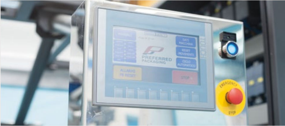
User friendly OMRON touch screen, with recordable programs menu system recipe based. Most of format changes and movements are electric and can be recorder and recalled. Machine can be operated from both sides, left and right machine with sliding or bifold doors
