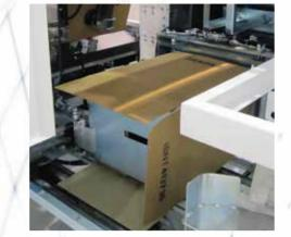
Positive motorized. Automatic cartons In feed conveyor with different loading Blank picking system provided with motor. opening and products insertion.
