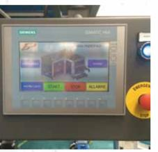
Machine controlled by Siemens PLC and intuitive touch panel. Auto adjustable change of format.
